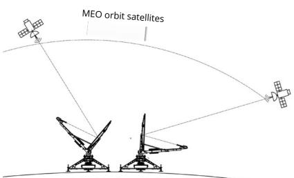
two terminals setup - synchronized to avoid interruption and without keyhole effect
